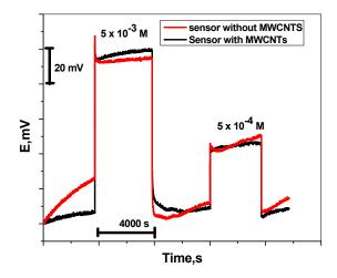
Figure 5. Water layer test for Tl membrane based sensor in the absence and presence of MWCNTs.
