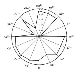
**Figure 4.** Selectivity coefficient (Log  $k_{Tl,J}^{pot}$ ) values of the proposed sensor using modified separate solution method (MSSM).
