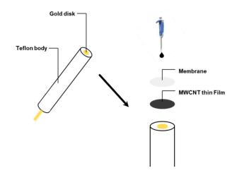
Figure 1. Sensor construction using multiwalled carbon nanotubes (MWCNTs)
