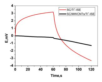
**Figure 6.** Chronopotentiograms for the solid-contact(SC/Tl<sup>+</sup>-ISE) (top) and SC/MWCNTs/Tl<sup>+</sup>-ISE (bottom) electrodes under the constant currents of  $\pm 1$  nA in  $1.5 \times 10^{-5}$  M of Tl<sup>+</sup> solution.
