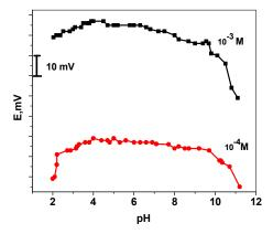
Figure 3. Effect of pH on the response of the sensor.
