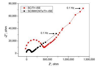
**Figure 7.** Electrochemical impedance spectroscopy (EIS)spectra of the SC/MWCNTs/Tl<sup>+</sup>-ISE with (circles) and SC/Tl<sup>+</sup>-ISE (squares) without the solid-contact layer of MWCNTs measured in  $1.5 \times 10^{-5}$  Tl (I) solution.
