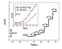
Figure 2. Time trace of the proposed sensors. Insert: Calibration curves of these ion sensors.
