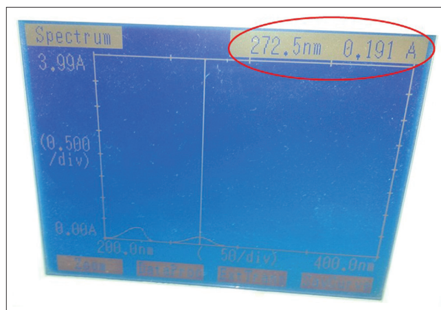
Figure 6: Determination of absorption maxima (lambda maximum) of zoledronate as displayed on digital screen of ultraviolet spectrophotometer
