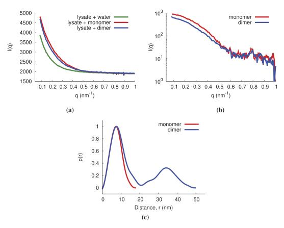
Figure 7. The scattering signal of monomers and dimers with a cell lysate background (separate capillary). (a) The dark-subtracted scattering intensity of a monomer and dimer solution and their background signal. (b) The subtracted scatter curves of the monomer and dimer solutions. (c) The p(r) of the monomer and dimer solutions.
