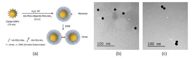
**Figure 2. Interaction model system.** (a) Schematic representation of the synthesis of the model system. TEM image of (b) monomers and (c) dimers, representing non-interacting and interacting species, respectively.
