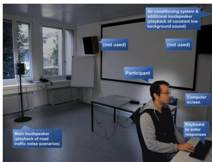
Figure 2. Photography of the laboratory setup (office environment at the Empa) used for the listening experiments. The loudspeaker positioned at the (closed) window mocked the road traffic noise scenarios at an open window, while the participant at a desk performed the visually presented cognitive task. The loudspeakers on the wall (left and right of the picture and indicated with “not used”) were not used in the current experiments. For details on the air conditioning system and the additional loudspeaker see Section 3.1.
