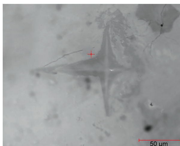
Fig. 3: Indentation on one of the samples postinfiltration
