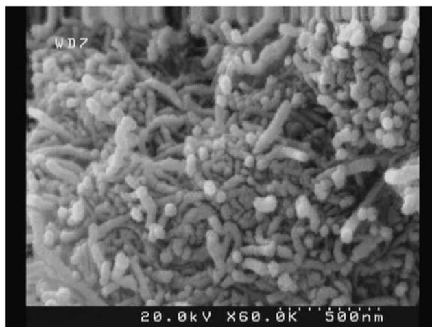
**Figure 4** SEM images of MWCNTs functionalized with INH.
