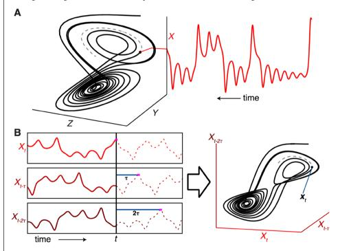
**Figure B1.** Reconstruction of System Dynamics from a Time Series (using the canonical Lorenz attractor example) (**A**) Projecting the motion of the Lorenz attractor onto the x-axis yields a time series for variable x. (**B**) Successive lags (with time step  $\tau$ ) of the time series  $x_t$  are plotted as separate coordinates to form a reconstructed (and visually similar) "shadow" attractor that preserves essential mathematical properties of the original system.
