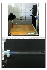
Figure 2: (a) Camera system, (b) small air bubble in 0.1 cc pipette of fluid filtration system
