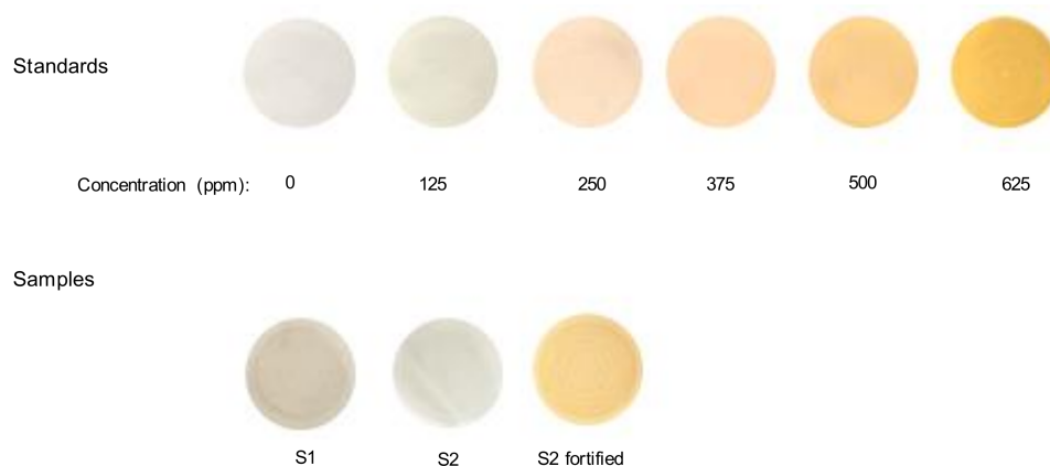
Figure 4. Images of the membranes obtained for the calibration solutions and for the drug-street samples.
