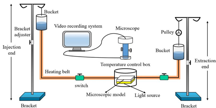
**Figure 1.** Microscopic visualization displacement experiment apparatus and process.
