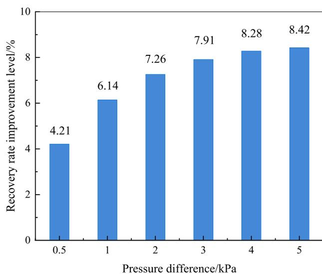
**Figure 12.** Influence of various pressure fluctuation amplitudes on the recovery rate (10 kPa pressure difference, 0.1 Hz frequency).
