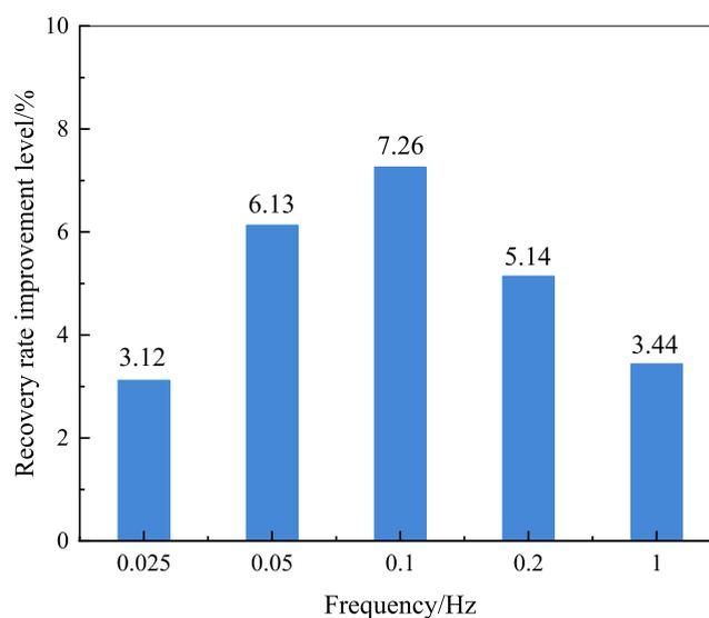
**Figure 13.** Impact of different pressure fluctuation frequencies on the recovery rate (10 kPa pressure difference, 2 kPa amplitude).
