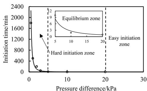
**Figure 3.** Start-up time under different pressure differences.
