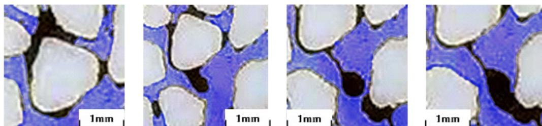
(b) The cluster-shaped and membranous residual oil
