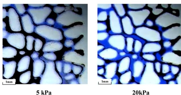
**Figure 8.** Distribution patterns of remaining oil under different pressure differences.
