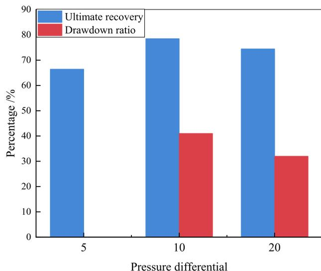
**Figure 10.** Recovery rates at different pressure difference and the proportion of elongation during high water-cut displacement.
