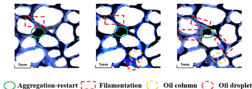
**Figure 9.** Process of aggregation, initiation, and displacement during the high water-cut period (microscopic elongation, oil droplets, and oil columns).
