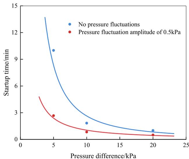
**Figure 4.** Impact of pressure fluctuations on start-up under different pressure difference (pressure fluctuation 0.5 kPa).
