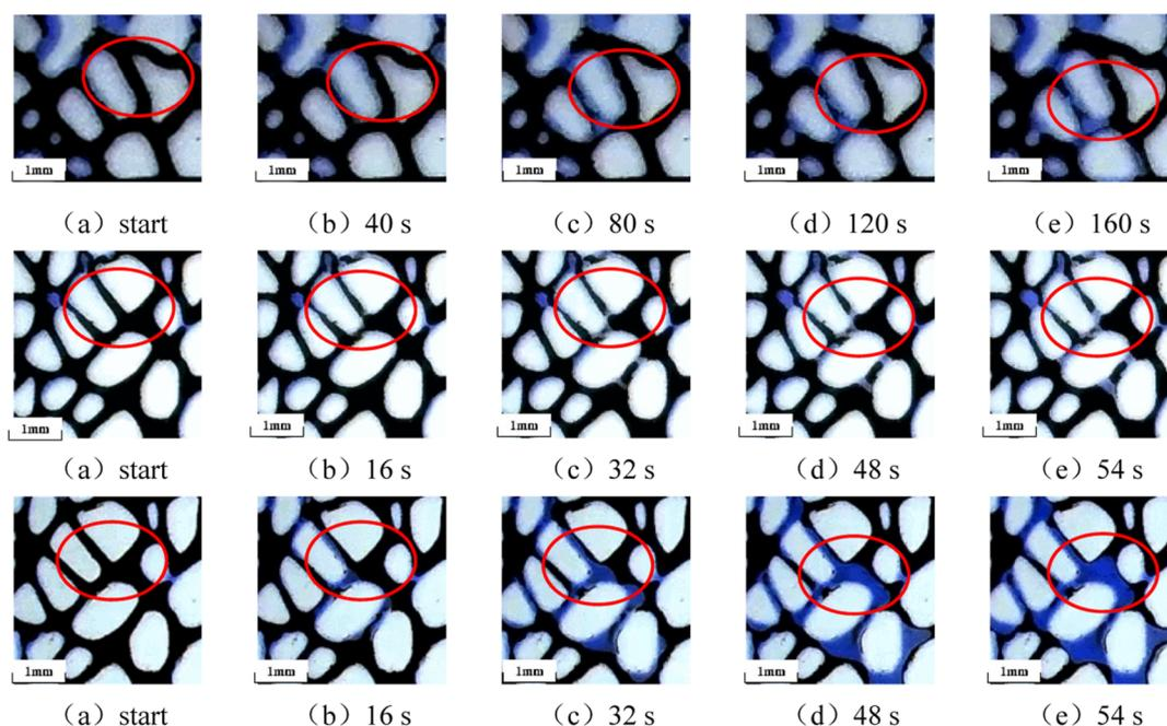
**Figure 7.** Process of water film thickening under different pressure differences (from top to bottom: 5, 10, and 20 kPa).
