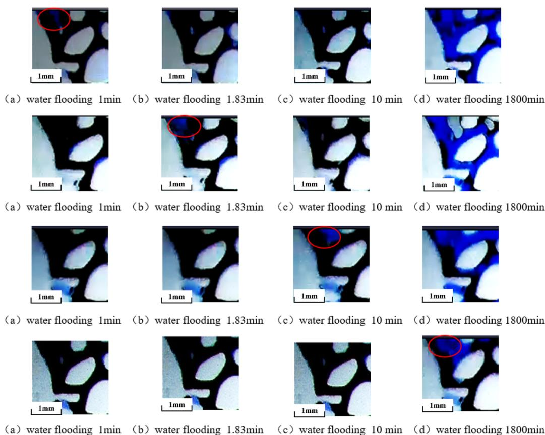
**Figure 2.** Initiation process of heavy crude oil under different pressure differences (from top to bottom: 20, 10, 5, and 0.5 kPa).
