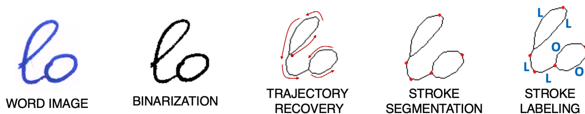
Figure 3. Each word image extracted from a document is processed by the query-by-string (QbS) retrieval system through the following steps: binarization [37], trajectory recovery [38], stroke segmentation [39] and, if a transcription is available for the word image, stroke labeling [40].
