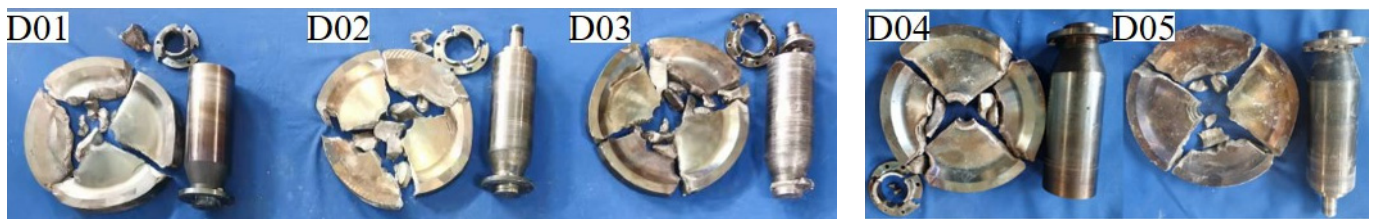
Figure 13. Discs after fatigue failure (D01–D05 are arranged from left to right).
