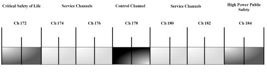
5.860 GHz 5.870 GHz 5.880 GHz 5.890 GHz 5.900 GHz 5.910 GHz 5.920 GHz
