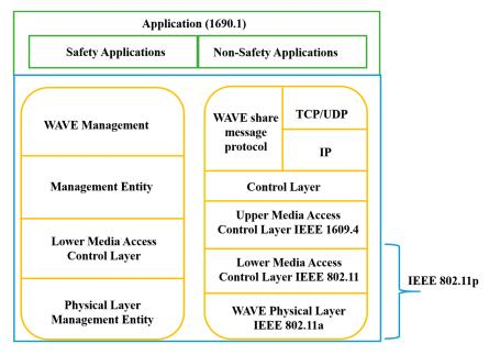
Figure 3. Wireless access in vehicular environments (WAVE) architecture.
