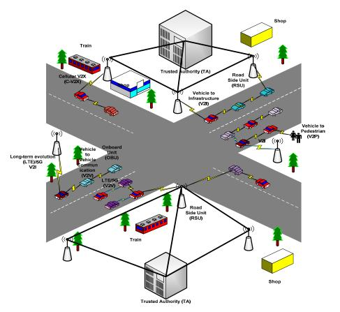
Figure 1. VANET model diagram.
