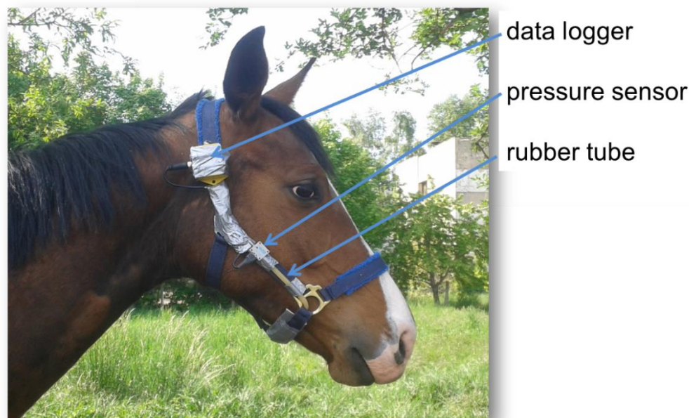
Figure 1. Modified halter equipped with measuring instruments for the detection of chewing parameters.
