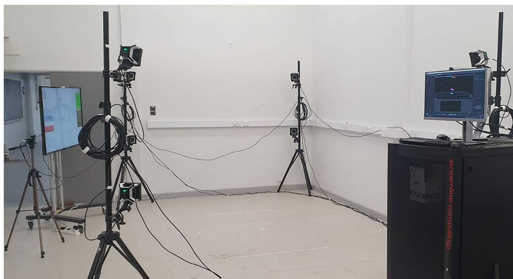
Fig. 8 The OptiTrack (marker-based) and NuiTrack (marker-less) capture environment used in the UL-RED data collection study. This follows the same layout description in Fig. 2. All cables were routed to ensure low risk to participants during entry to and exit from the capture arena. The capture area was situated in a closed room with no direct sunlight to ensure minimal interference to both the marker-based and marker-less systems.
