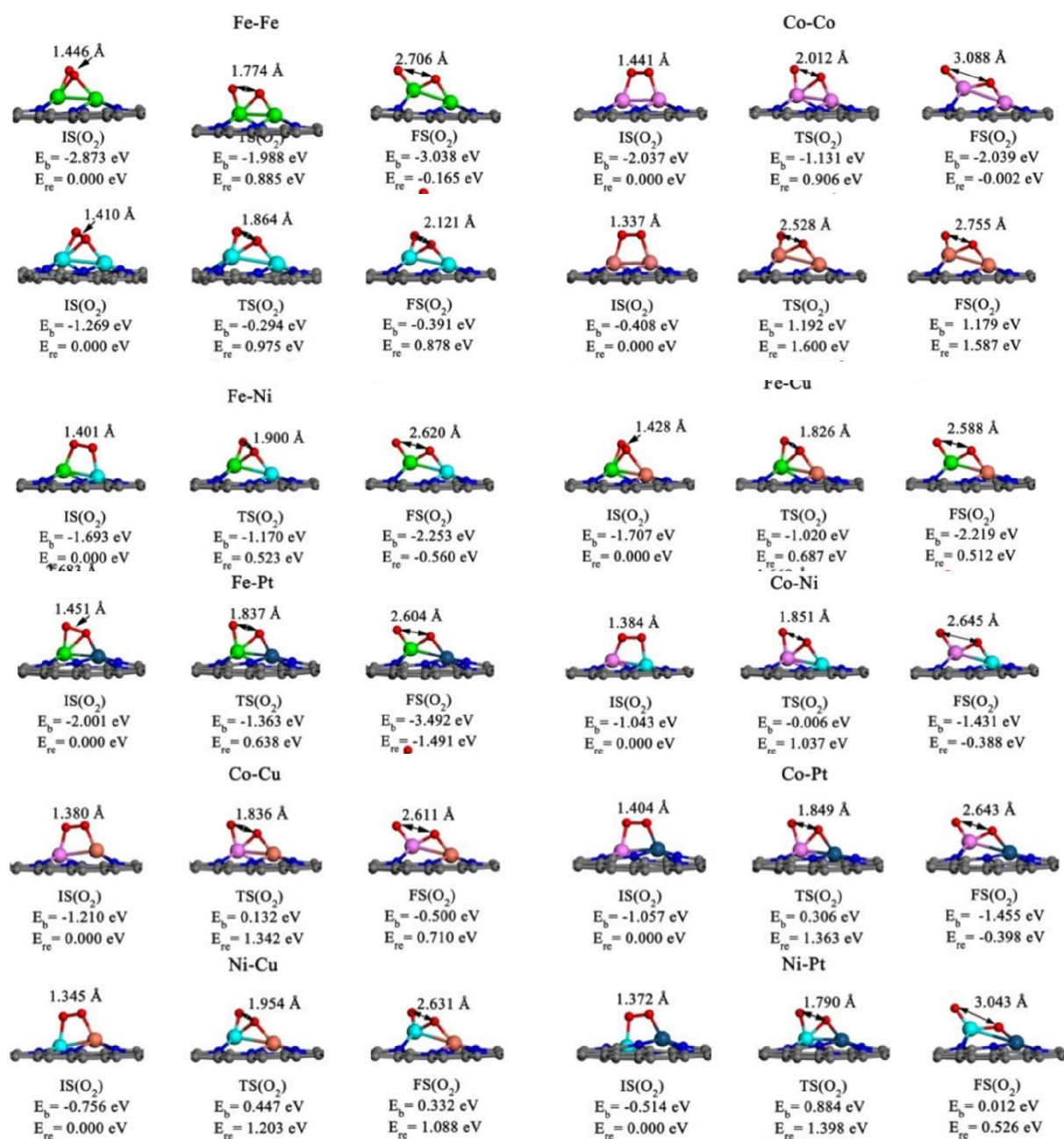
Figure R18. Optimized structures, binding energies ( E_b ) and relative energies ( E_{re} ) of the O_2 activation on different M_1N_3 - M_2N_3 @NGr structured DACs. IS: initial state; TS: transition state; FS: final state. The O atoms in adsorbates are all represented by red spheres. [Reprint (adapted) with permission from Chuanyi Jia, Qian Wang, Jing Yang, et al., Toward Rational Design of Dual-Metal-Site Catalysts: Catalytic Descriptor Exploration, ACS Catal. 12, 3420–3429 (2022). Copyright © 2022 American Chemical Society.]
