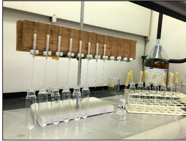
Fig. 6. – Sample extracts being eluted through acidified silica gel columns and collected in TurboVap® tubes.
