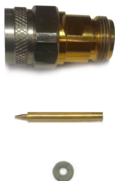
Figure 1. Coaxial transmission line (on top) with a central conductor (in the middle) and a composite sample (at the bottom) for microwave measurements.
