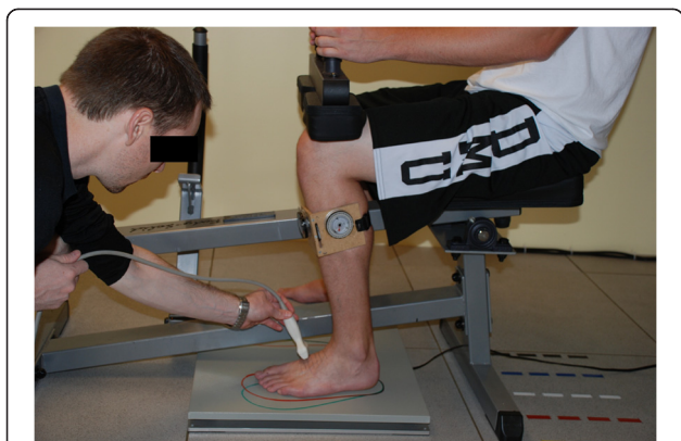
Figure 2 In-house modified calf raise apparatus with force plate under the loading pad. Subject's knee and ankle are both flexed at 90^\circ with the tibia perpendicular to the ground. The 0^\circ and 15^\circ abducted footprints can be visualized as well as the parallel lines drawn on the dorsum of the subject's foot parallel to the Lisfranc ligament.
