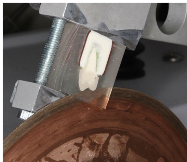
Figure 15. Cold cured acrylic blocks sectioned with diamond discs attached to a cutting machine.
