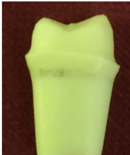
Figure 4. Original Frasco prepared teeth of each group were marked 2 mm apical to the cemento-enamel junction circumferentially.
