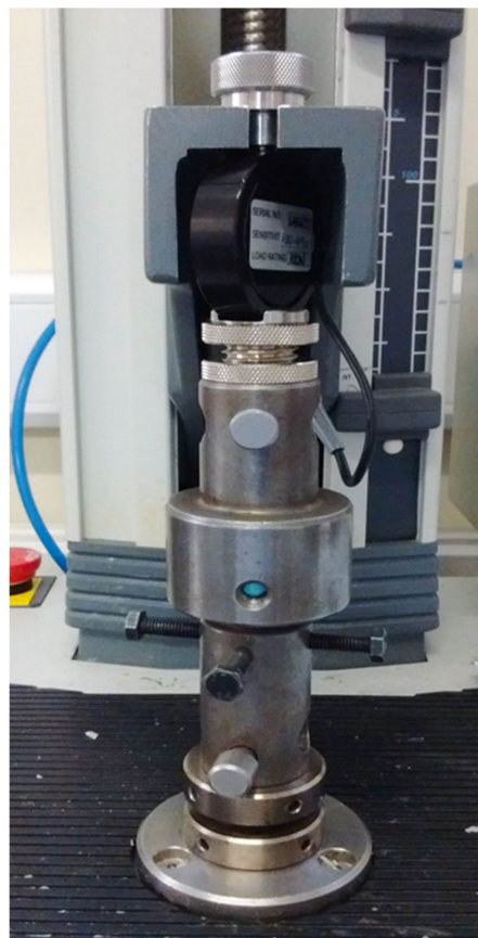
Figure 11. Final cementation settings by using the tensometer.
