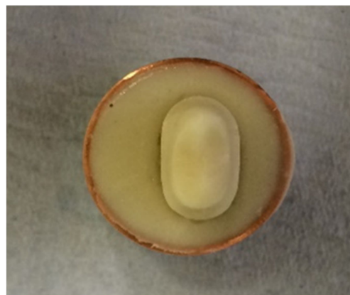
Figure 10. Addition light body silicon impression material (President Plus ® ) injected and reinserted to simulate periodontal ligament.
