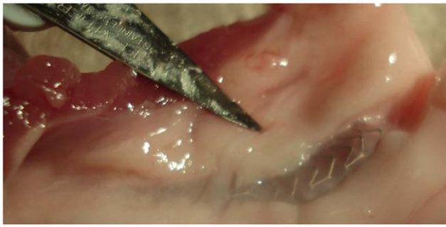
Figure 1. ML Frontier™ stent in porcine coronary artery. Immediately after excisement the ML Frontier™ stents were implanted in fresh vascular bifurcation tissue in the porcine heart samples. doi:10.1371/journal.pone.0021778.g001
