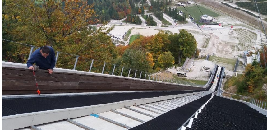
Figure 10. Measurements with the single-prism method on the inrun of Planica ski-flying hill.
