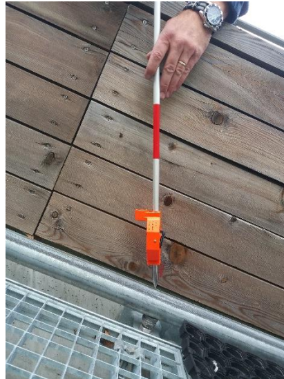
Figure 3. Measurement with the Leica GMP111-0 mini prism.
