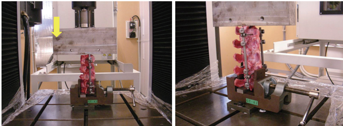
Fig. 4. The instrumented lumbar spine was axially compressed by using the surface of a rectangular platform of an AG-X testing machine.
