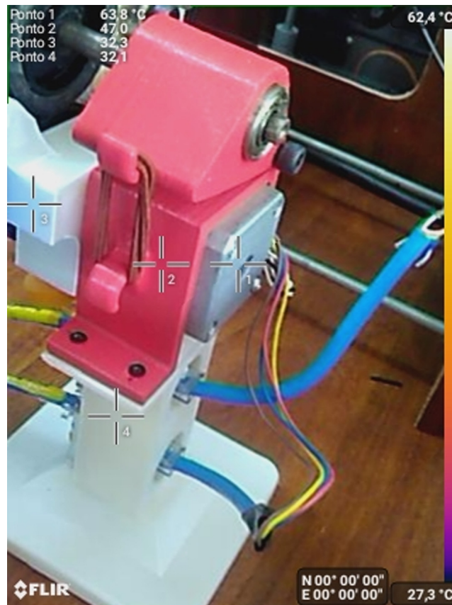
Fig. 10. Thermal analysis of the puller system during the process.
