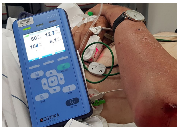
Fig. 1 ICON connected to a patient. Size and weight of this device size, weight (20 cm × 10 cm × 4 cm; 1.36 kg). Display shows heart rate, cardiac output, cardiac index and stroke volume. SQI can be seen as green bars in the top left of the screen
