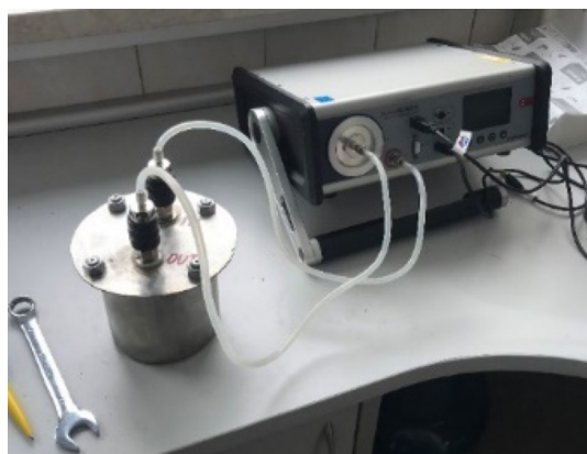
Figure 2. Set up for radon accumulation measurements for assessment of the emanation coefficient in the laboratory environment. Set include the small accumulation chamber with the total volume of 0.00114 \text{ m}^3 (present on the left side) operating with the AlphaGuard instrument (presented on the right).
