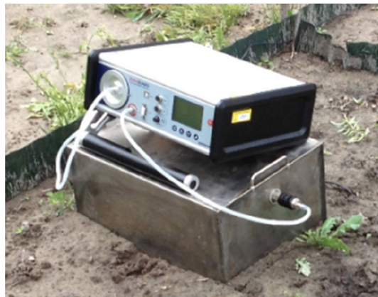
Figure 3. Setup for assessment of the radon exhalation rate in the field measurements. The set consist of the accumulation chamber with 0.024 m 3 in volume and the AlphaGuard instrument.
