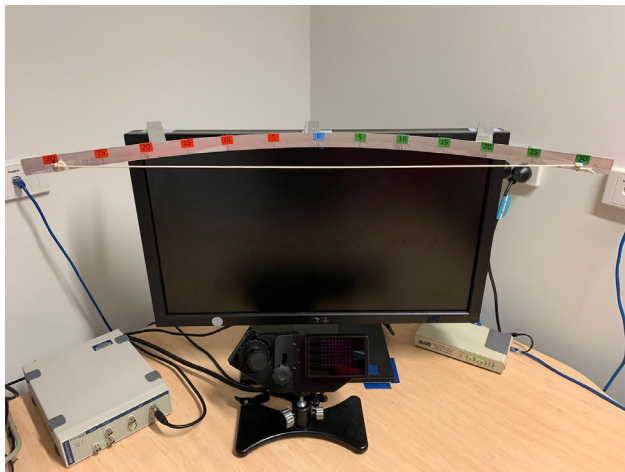
FIGURE 1. A metal arc mounted to the top edge of the monitor with targets at \pm 30^\circ from the center in 5^\circ steps. It was used to measure the gaze position of the subject.
