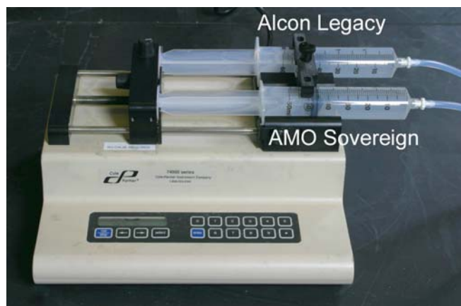
Fig. (2). Controlled irrigation flow was delivered to the phacoemulsification probes using a Cole Palmer dual syringe pump.
