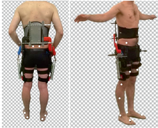
FIGURE 7: Placement of the markers according to the lower body plug-in-gait marker-set. Markers are placed on the pelvis (ASIS and PSIS), thigh, knee, shank, ankle, heel, and toe.
