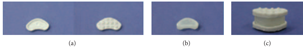
FIGURE 2: The parts and the whole of the disc prosthesis. (a) Two sides of HAPEX endplates, (b) composite hydrogel for IVD substitute, and (c) total IVD substitute prototype [11].
