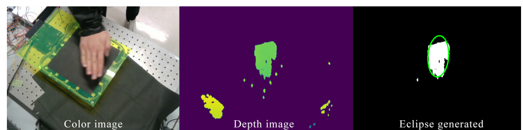
Figure 11. Hand position recognition process using depth camera.
