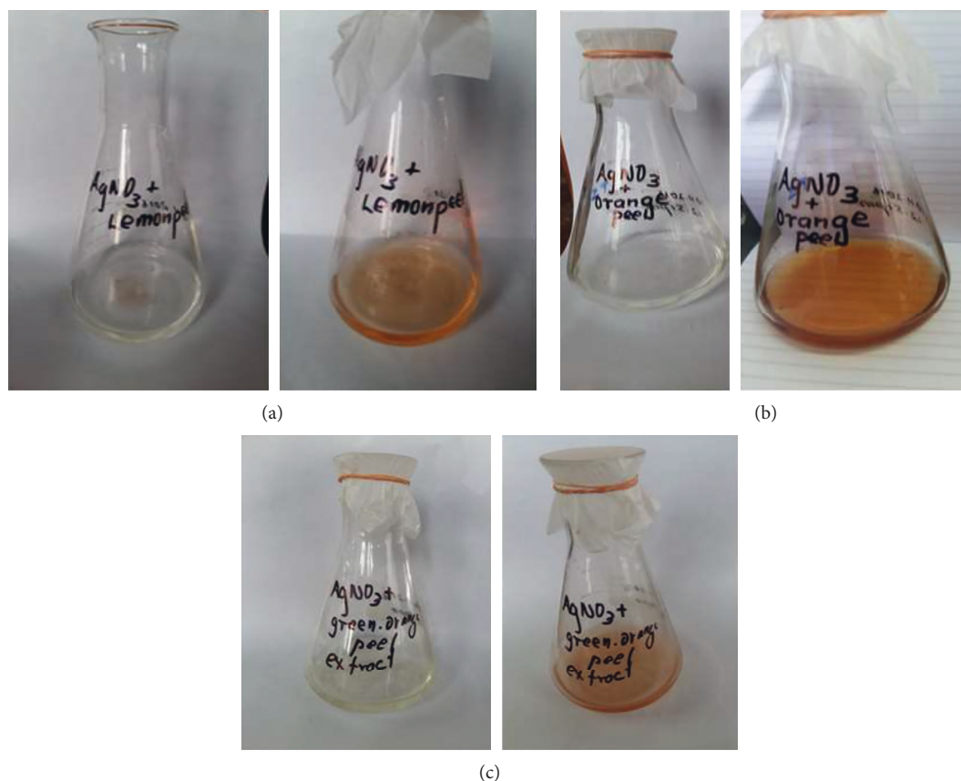
FIGURE 1: Colour change in the solution after the addition of (a) lemon peel extract, (b) orange peel extract, and (c) green orange peel extracts due to reduction of silver ions.
