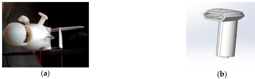
Figure 4. The hoods where the temperature and humidity sensors are placed: (a) hoods installed on the top of OVLI-TA fuselage; and (b) 3D design of the hoods.
