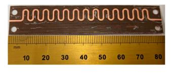
**Figure 3.** Top view of the proposed periodic 13 unit-cell antenna fabricated on 0.254 mm thick grounded Arlon DiClad 880 substrate. (a) Geometry. (b) Prototype.
