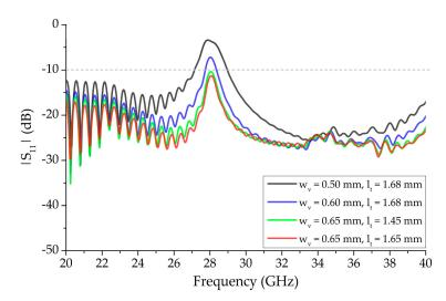
**Figure 5.** Effect of varying vertical bowtie segment parameters,  $w_v$  and  $l_t$ , of 13 unit-cell element periodic structure independently on  $|S_{11}|$  while the other parameters remain the same as Table 1.
