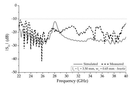
**Figure 8.** Simulated and measured  $|S_{11}|$  of 13 unit-cell element periodic structure with bowtie vertical unit-cell segments.
