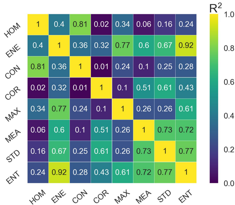
Figure 3. Heat map of the inter-feature correlations. The values show the coefficient of determination ( R^2 ).
