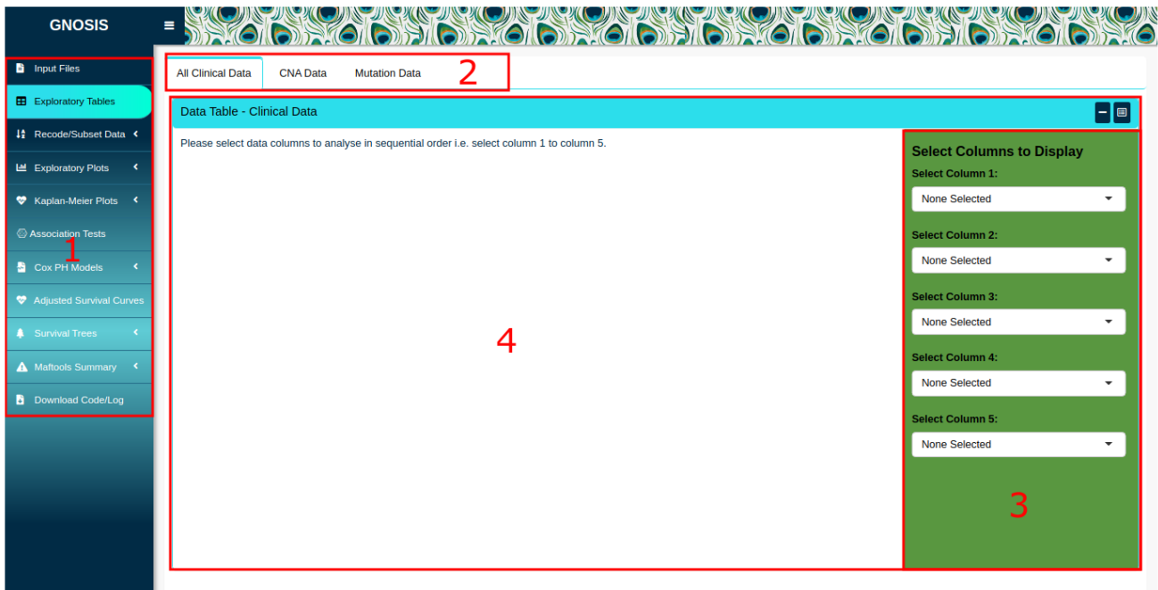
Figure 1. GNOSIS GUI with highlighted interface elements. (1) The Exploratory Tables tab is selected in the tab sidebar. (2) Within tab panels allowing multiple operations to be carried out and viewed in the one tab. (3) Box sidebar allowing users to select inputs, alter arguments and customise and export visualisations. (4) Viewing panel displaying output.
