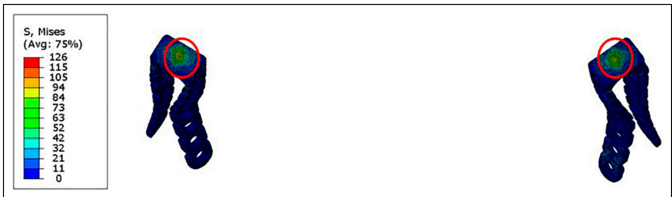
Figure 9. Stress distribution and peak stress locations on the plates in the fork plate system during 10Nm flexion motion and 400N preload.
