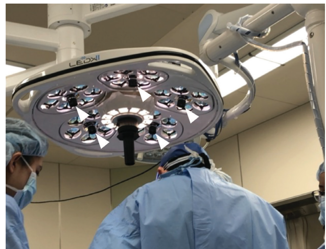
Fig. 1. The overhead multiview camera system integrated into a mobile stand type operating room light. The center LED of each light module was replaced with CCD camera (arrowheads), creating a situation in which at least one camera shoots the surgical field when light from any of the LEDs reaches surgical field.
