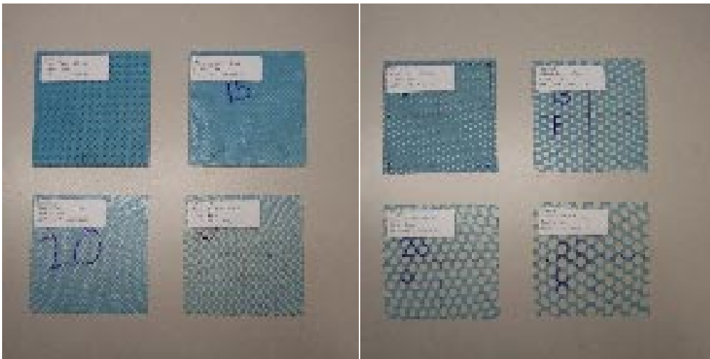
FIG. 1. Photographs of the mask samples measured in this investigation. The photo on the left is the material with the smaller holes, and the photo on the right is the material with the larger holes. The material was stretched different amounts in a reproducible way.
