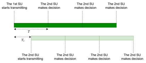
**Figure 4.** The communication mechanism in asynchronous Transmit-Receive (TR) mode. A delay of  $T_s$  is made in order to reduce the collision time between the secondary and the primary transmissions.
