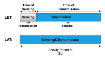
**Figure 2.** The two main functioning modes of SU activity. Listen-before-Talk (LBT): SU remains silent during the sensing period and no sensing is performed during the transmission. Listen and Talk (LAT): sensing and transmission are made concurrently.
