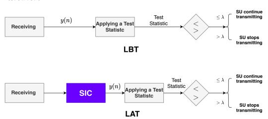
**Figure 3.** Spectrum Sensing processes under LBT and LAT. For LBT, no Self-Interference Cancellation (SIC) module is required since there is no simultaneous Transmit-Sense (TS), and the Test Statistic may be directly applied to the received signal. By contrast, SIC is applied before evaluating the Test Statistic in LBT to reduce the effect of SI on the Spectrum Sensing (SS) performance.
