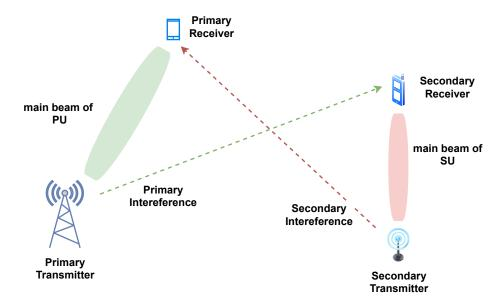
**Figure 5.** Spatial Dimension of CR application: SU is able to exploit the spatial dimension by transmitting in a non-overlapping direction with the PU transmission. Here, SU should be able to estimate/know the PU beam in order to avoid the interference.
