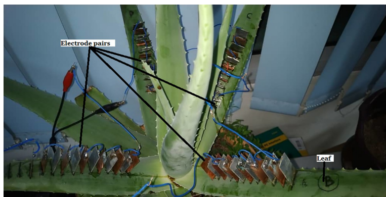
Fig 9. Experiment setup for series connection among leaves in which the connection by-passes the stem of the Aloe Vera.
