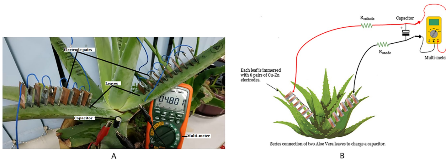
Fig 13. Experiment setup for charging a capacitor using the PBC system. Example of setup arrangement (A) and simple schematic of the setup (B).
