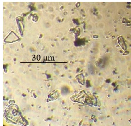
Figure 4. Micrographs of the mechanical mixture of \text{H}_2\text{SO}_4 -doped PANi (20 wt.%) and talc (80 wt.%).
