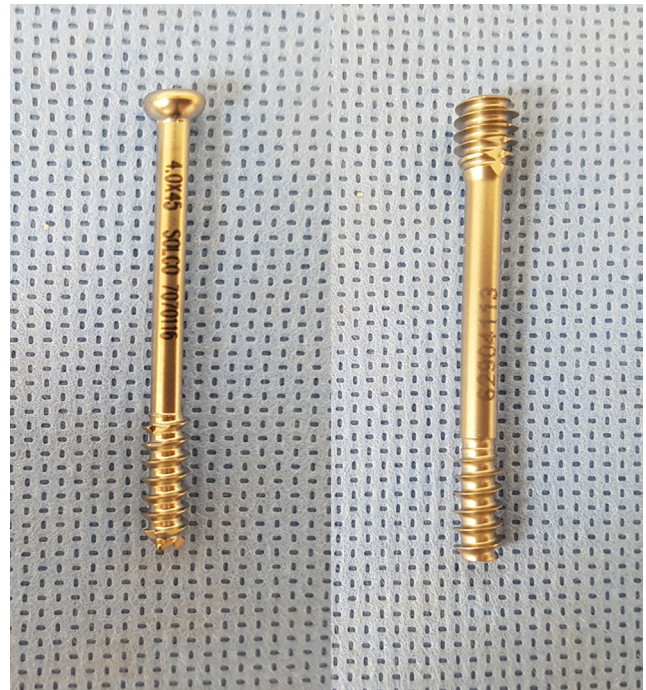
Fig. 1. Showing the studied implants; the 4.0-mm cannulated cortical screw (left) and the 4.5-mm headless compression Herbert screw (right).
