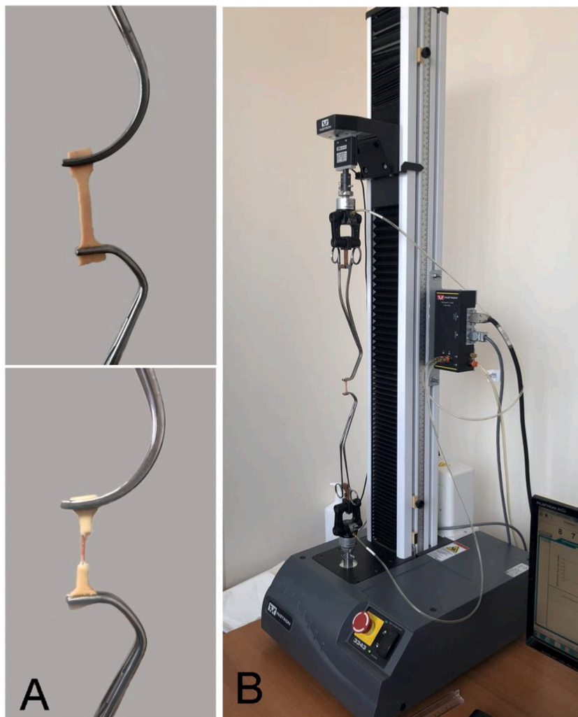
Fig. 2. (a, b). The mechanometric testing of aortic tissue sample. A—Tissue sample of the ascending aorta, fixed in atraumatic clamps. B—Instron 3343 testing machine with a sample of aortic tissue.
