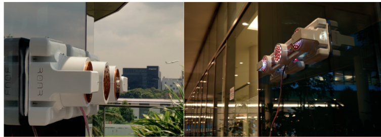
Figure 1. A situation in which the Mantis cleans a glass window panel of a building.
