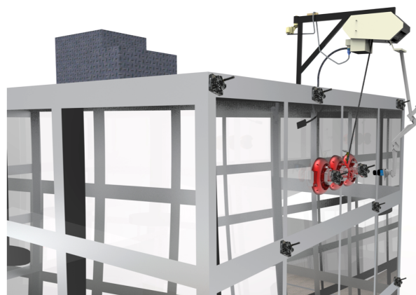
Figure 9. Beacon navigation system terminals on the glass façade structure of a building, in strategic corners of the windows.
