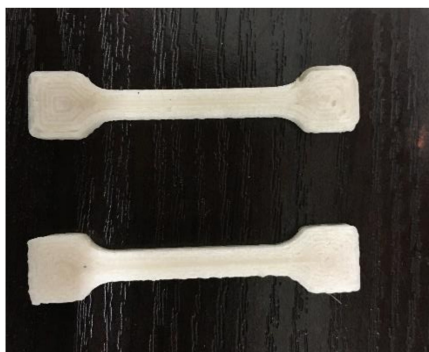
Figure 1. Printed specimens of ABS/octyl-QDED for tensile tests.
