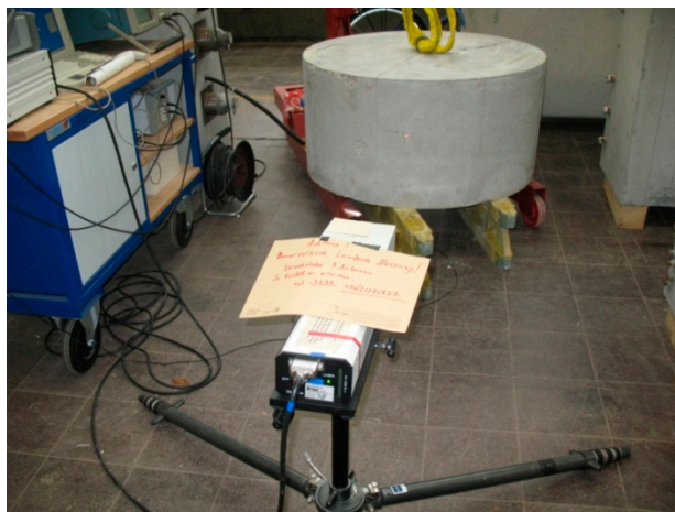
Figure 6. Experimental setup for measurement of directivity patterns. Transmitting transducers are embedded in the center of the concrete block. Surface movements are recorded by a laser vibrometer (in front).
