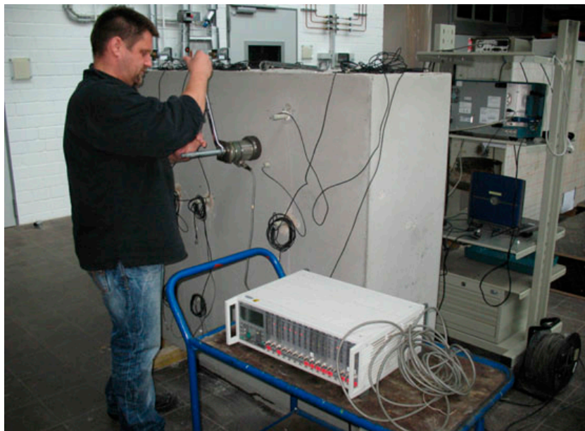
Figure 10. Concrete specimen GK32 with embedded transducers and load application system. From [26].
