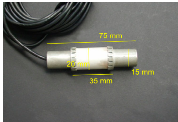
Figure 1. Photograph of the novel ultrasonic transducer for embedment in concrete (Manufacturer: Acsys Ltd., Moscow, Russia. Photo: BAM).
