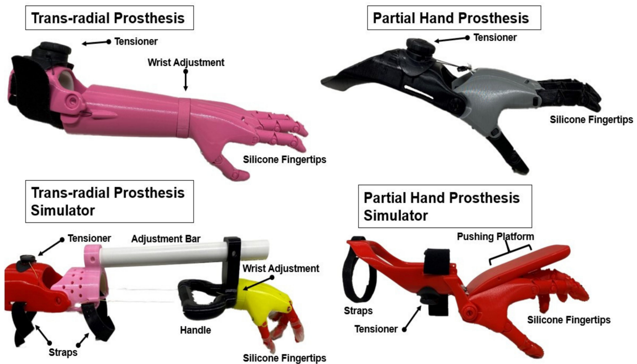
Figure 1. Description of prostheses and prosthetic simulators. The prosthetic simulators used in the study mimic the design and control mechanism of the prostheses. The partial hand prosthesis simulator allowed TD children to rest their existing hand on top of the simulator hand, with the wrist in slight extension. A pushing platform placed above the hand allowed active wrist flexion and passive extension to facilitate actuation of the hand. Similarly, the trans-radial simulators incorporated similar features to the trans-radial prosthesis, with the addition of a handle that allowed typically developed children to actuate the device by elbow flexion.
