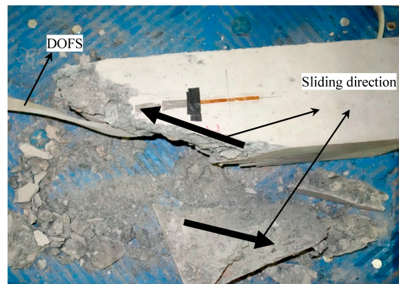
Figure 16. The concrete column after failure.
