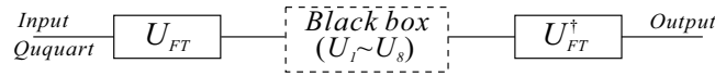
Figure 1. Quantum circuit to realize the permutation algorithm. U_{FT} denotes the Fourier transformation. The black box contains all the eight permutation operators in the algorithm and U_{FT}^\dagger is the inverse Fourier transformation.
